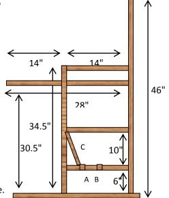
The two additional horizontal 1.25" x 0.75" on the horizontal at 6" above the base, at 4.5" (A) and 8.5" (B) from the rear are referred to further in 3. below. The one furthest forward provides support for the front 6mm ply board (C) which is angled in, directed backwards, at its lower edge.
